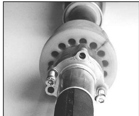
FIG. 58: 2 SCREWS USED AS JACK SCREWS
