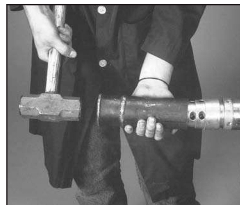
FIG. 31: USING PIPE TO SECURE STEPPED CONE
