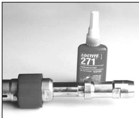
FIG. 51: APPLY LOCTITE AND TIGHTEN CONTROL STUD ADAPTER
