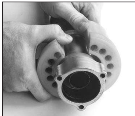
FIG. 69: PLACING ELASTIC BLOCK ON CONTROL TUBE
