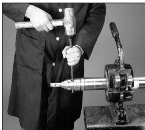
FIG. 20: REMOVING THE ROLL PINS
