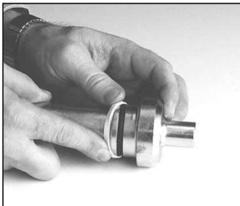
FIG. 25: SLIDE CHISEL SEAL ONTO CHISEL
