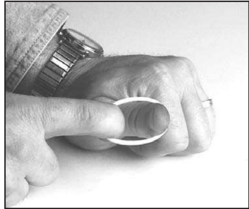
FIG. 46: STRETCH NEW SEAL TO FIT CONTROL STUD
