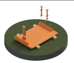
2. Spin out Spindles to the required length and position into the channels alternating as shown. Secure using Pins & R-Clips as shown in Detail A.
