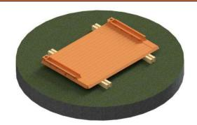
1. Lay Drag Box panel down on a level surface on suitable timber bearers using the 4-Leg chain provided.
