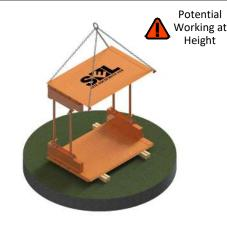
3. Lower opposite panel onto spindles using the 4-Leg chain. Chain hooks to be secured to the handling points at the upper and lower ends of each channel. Secure to spindles using Pins & R-Clips. Do not remove slack in the chains until all the spindles are secured.
