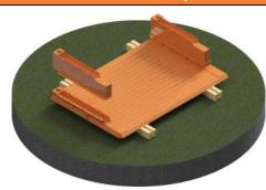
1. Lay Manhole Box panel down on a level surface on suitable timber bearers using the 4-Leg chain provided. Secure the lifting hooks through the handling points at the upper and lower ends of the channels. Connect the Manhole Profiles using 8no M20x40 bolts per
