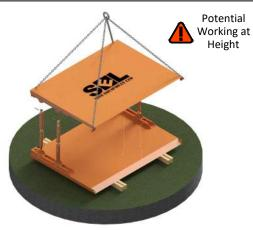
2. Lower the opposite panel onto the spindles using the 4-Leg chain. Chain hooks to be secured to the handling points at the upper and lower ends of each side. Secure to spindles using 20Ø Pins & R-Clips. Do not remove slack in the chains until all the spindles are secured.
