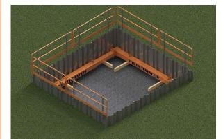
6. Lay timber bearers down within the excavation and using suitably load-rated lifting chains, lift the entire frame level into the excavation. Slightly pump in the legs to ensure ease of installation. Once installed to the correct level, pump out to the required size and install the restraint chains. Ensure lock off valves are engaged Do not use the restraint chains for lifting.
