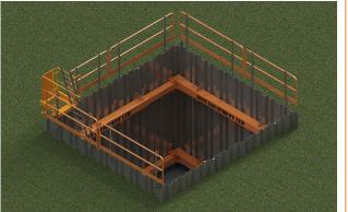
7. Excavate to the next frame level (as per TWD) and repeat Stage 6 with the next, and any following frame levels. When lifting an assembled frame level down, ensure that it is retracted sufficiently to fit between the upper frames. If this is not possible, install leg by leg within the excavation. Ensure suitable edge protection is installed, leaving a digging window if required.
