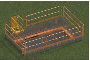
7. Ensure that all the sheets are pushed to their final levels, normally the formation level. Install suitable access and edge protection system. The removal of the equipment is the reverse of this procedure, reinstalling the temporary frame levels where required as backfilling progresses.
