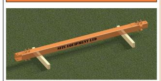
1. Lay first Double Acting Brace leg down on level ground on suitable timber bearers. Connect lifting hooks through the lifting points on the outer body. If preffered, the legs can be assembled within the excavation at the level specified in the Temporary Works Design. Follow steps 1-3 within the excavation.
